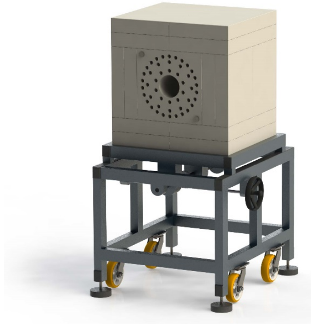
Figure 4. 3D view of the BELEN-48 detector polyethylene moderator matrix placed on its supporting structure. The ^3\text{He} counters will be inserted in the small holes located around the big central hole.
