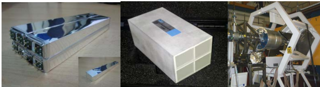
Figure 15. Left: Picture of a bunch of 4 Cs(Tl) (22 cm long) wrapped with VM2000 and couple to the customized LAAPD (S- 8622 of Hamamatsu). Central: Picture of a bunch of four \text{LaBr}/\text{LaCl} phoswich (St. Gobain). In this prototype the first stage has a length of 4cm and the second one of 6 cm. Left: Several experiments in-beam have been performed using CsI(Tl) and \text{LaBr}_3/\text{LaCl} units in its DEMONSTRATOR version
