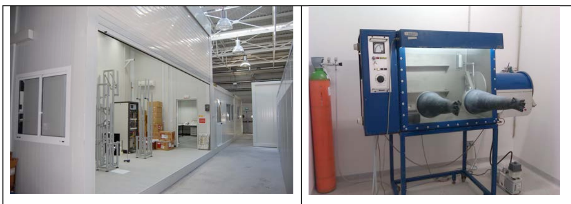
Figure 11. Left: photo of the new facility for the MONSTER assembly and test at CIEMAT. Right: photo of glove box room for the mounting/filling of the liquid scintillators in N 2 atmosphere.
